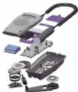
Figure 4: Exploded diagram of wind-up Freeplay Fetal Heart Monitor
