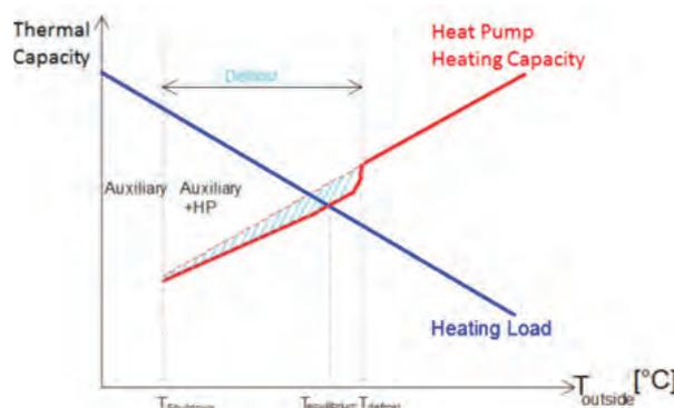
Figure 11: Operation of a heat pump in heating mode
