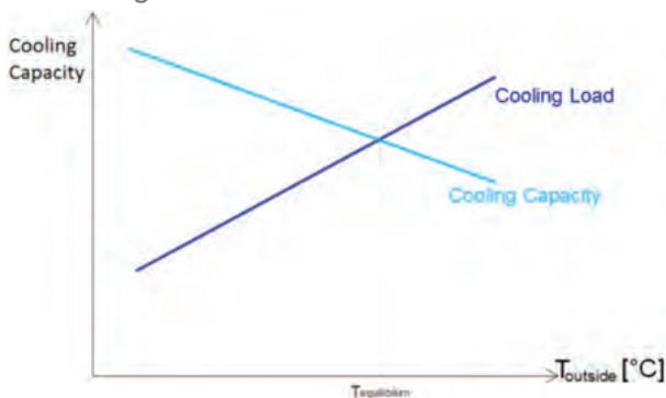
Figure 13: Operation of heat pump in cooling mode
