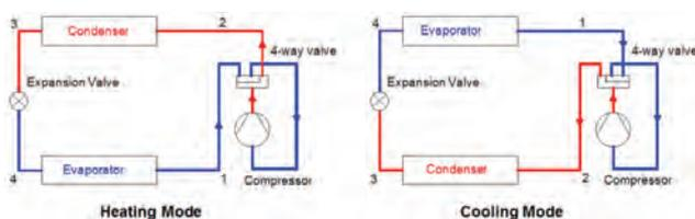
Figure 2: Reversing the cycle from heating mode to cooling mode by a 4-way valve (Kinab, 2009)
