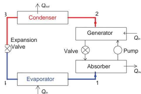
**Figure 9: Absorption heat pump**
