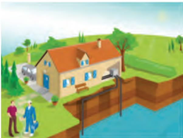
**Figure 8: Ground source heat pump (AFPAC, 2013)**
