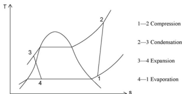
Figure 3: Thermodynamic vapor compression cycle (Temperature – Entropy diagram) (Kinab, 2010)
