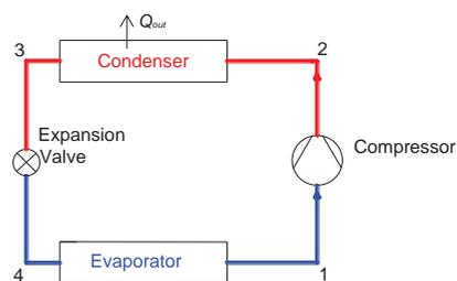
Figure 1: Heat pump components
